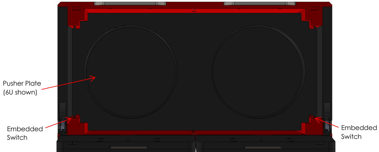
Figure 14: Deployment Confirmation Switches
